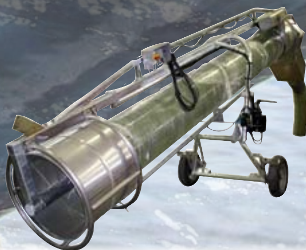
77 Class Ø 550mm 6,5m long fishing elevator.
