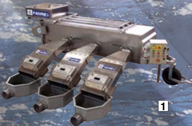
Helios 30 Grader fitted with 3 counters
